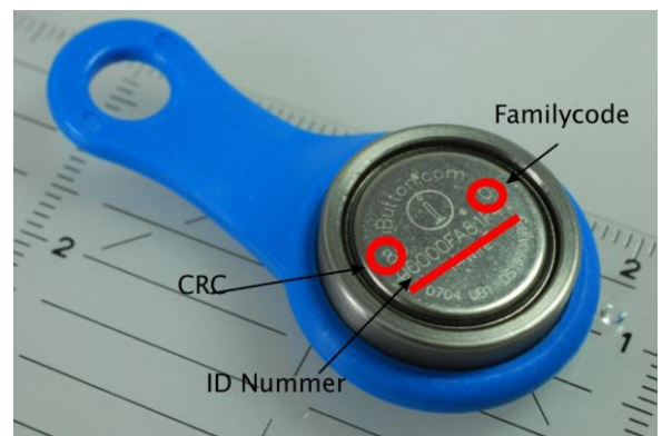
Figure 4: Meaning of lasered labeling of the key
